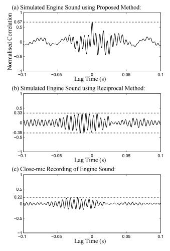
Figure 4. Normalised cross-correlation of the recording of engine at position  $\mathbf{B}$  with (a) the auralised sound at the same point using the proposed method (b) the auralised sound using the reciprocal method and (c) the unprocessed recording of engine at position  $\mathbf{A}$ .
