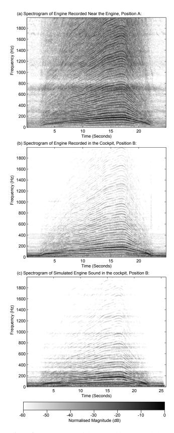
**Figure 3**. Spectrograms of the car engine (a) recorded at position **A**, (b) recorded at position **B** and (c) auralised at position **B** using the recording at position **A** as the source.
